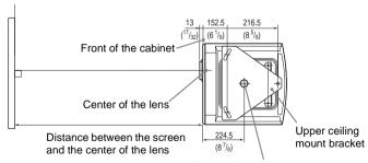
Center of the supporting pole (The center of the supporting pole is different from that of the unit.)
