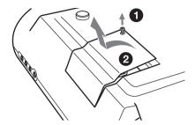
4 Loosen the three screws on the lamp unit with the Philips screwdriver 1. Pull out the lamp unit by the handle 2.
