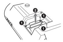
5 Insert the new lamp all the way in until it is securely in place 1. Tighten the three screws 2. Fold down the handle.
